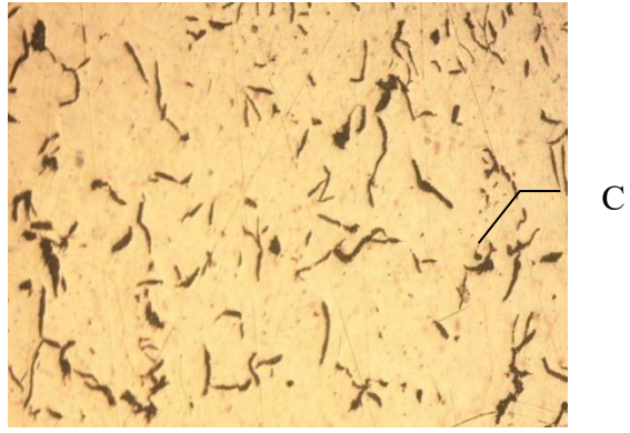
Picture 6 – Microstructure of the primary cast iron section
